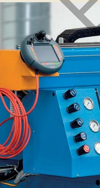
▶ Mobile touch panel is an optional solution for the machine operation control
