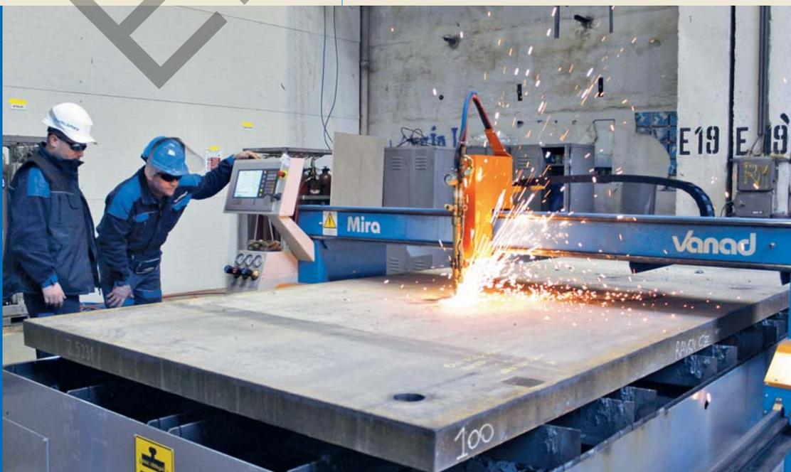
◀ The CNC cutting machine Vanad MIRA is equipped with oxy-fuel technology, laser pointer and electric flame ignition of the oxy-fuel torch. The picture shows the piercing of 100 mm structural steel. The CNC machine MIRA is also installed in our showroom, where you can see and try it
