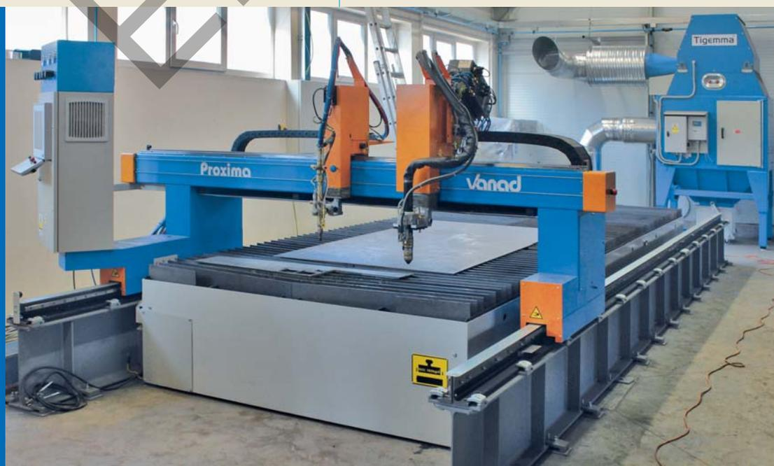
◀ Comprehensive cutting station PROXIMA built in 2014. CNC cutting machine is equipped with the Kjellberg HiFocus 360i plasma system, oxy-fuel technology, Tigemma filter system and Orlik compressor
