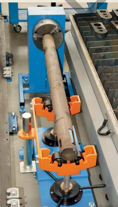
◀ Positioning and the detail of the supplementary device RotCUT for the SUPREMA cutting machine
