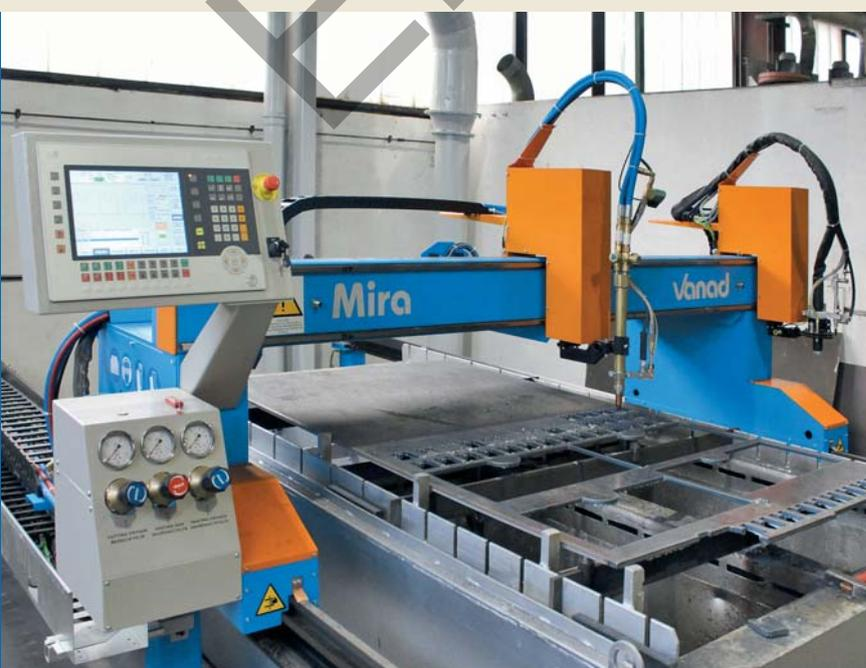
◀ The Vanad MIRA cutting station built in 2013 with the Hypertherm Powermax 105 plasma system
