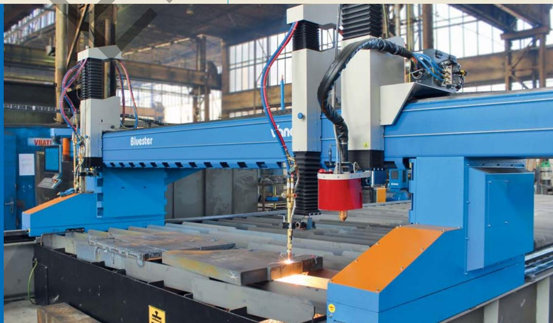
◀ Cutting station BLUESTER 45 x 120 built in 2014 with the Kjellberg HiFocus 440i plasma system and oxy-fuel technology
