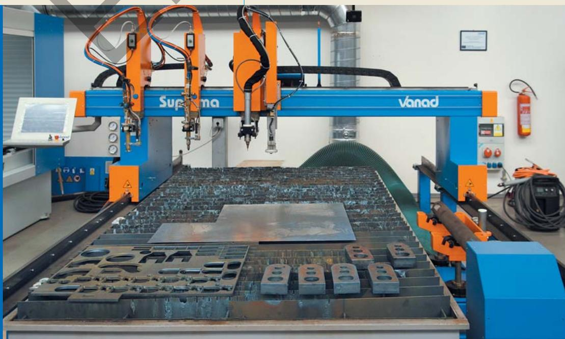
◀ SUPREMA cutting station built in 2014. The CNC cutting machine is equipped with the Hypertherm Powermax 125 plasma system and oxy-fuel technology.
